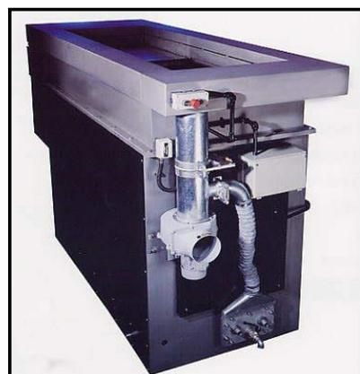
Figure 2. Tank for degreasing in the vapor phase.
