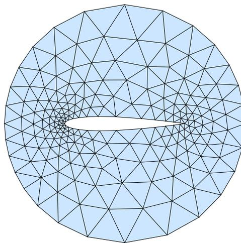
**Figure 3.** Example of nonuniformly generated mesh: the airfoil.
