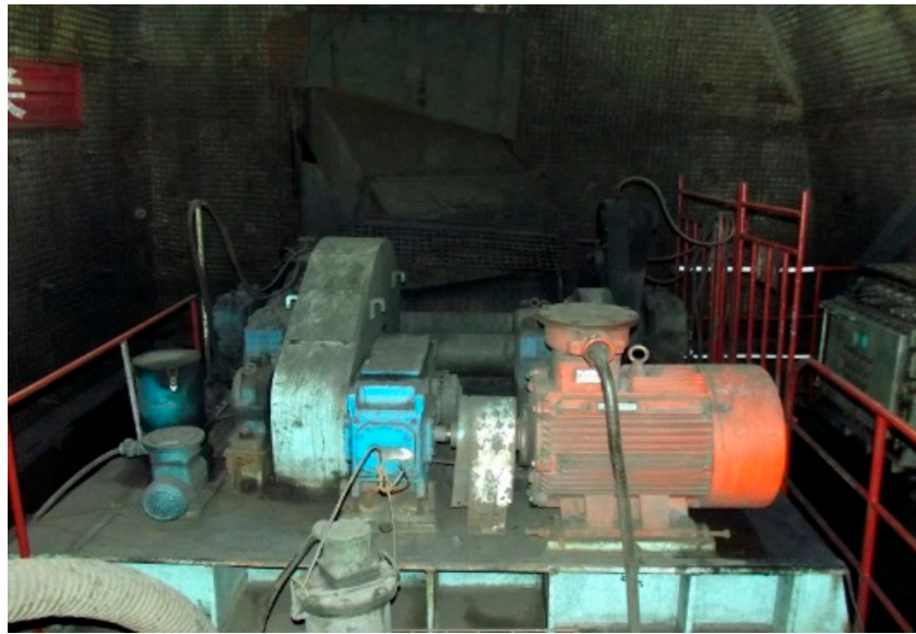
Figure 3. The new driving system of the underground mechanical moving sieve jig.
