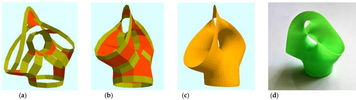
**Figure 17.** Modeling *Single-Sided Interruption*: (a) a skeleton with a Möbius ribbon on top; (b) the connecting mesh; (c) the subdivision surface; (d) a resulting 3D printed model.
