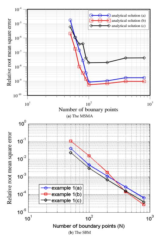
**Figure 8.** Comparison of the accuracy with the MSMA and the singular boundary method (SBM): (**a**) the MSMA and (**b**) the SBM.
