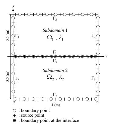
Figure 17. Boundary and source points for the example with two layered materials.
