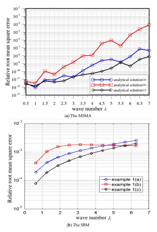
**Figure 9.** Accuracy comparison for the relative root-mean-square error versus the wave number: (**a**) the MSMA and (**b**) the SBM.
