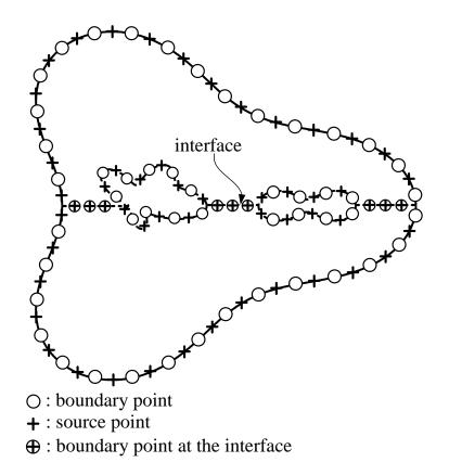
Figure 14. Collocation points for the example bounded by a multiply connected domain.
