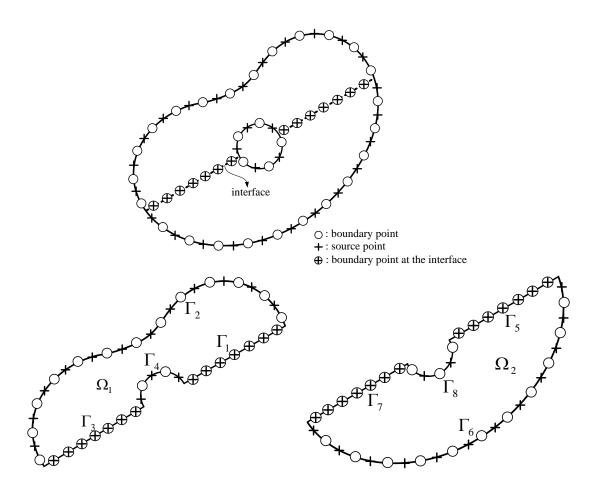
Figure 2. Diagram of the domain decomposition method (DDM) in a doubly connected region.
