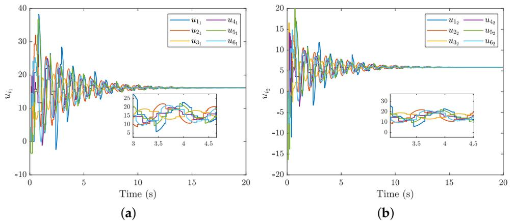
**Figure 4.** Profiles of control inputs  $u_i$  of the agents under our proposed algorithm. (a) Profiles of the control inputs  $u_{i_1}$ . (b) Profiles of control inputs  $u_{i_2}$ .
