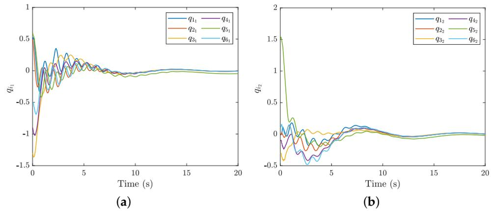
**Figure 2.** Profiles of agent positions under our proposed algorithm. (a) Profiles of agent positions  $q_{i_1}$ . (b) Profiles of agent positions  $q_{i_2}$ .
