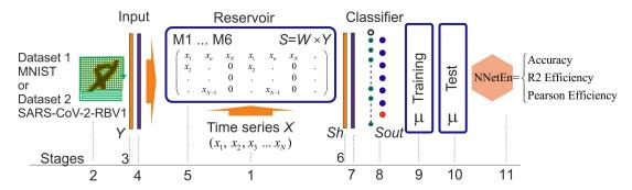
**Figure 3.** Main steps of NNetEn calculation [1]. The figure shows the main stages of calculation NNetEn based on the reservoir neural network LogNNet, where the reservoir is filled with the time series under study, and the entropy value is proportional to the classification metric of the reference database.
