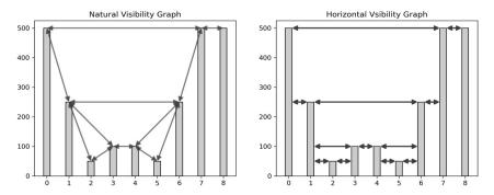
**Figure 2.** Illustrative example of the natural visibility graph representation for a time series (**left**) and the horizontal visibility graph representation for the same time series (**right**). The arrows in the images explains the projection of the visibility horizon when constructing the graph.
