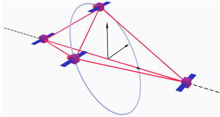
**Figure 1.** Tetrahedral formation. Four satellites in the orbital reference frame maintain a tilted tetrahedron. Over the motion around the Earth, the tetrahedron rotates, and two satellites move along the same orbit (dashed black) with a constant shift. Two other satellites rotate in the orbital frame, moving along a blue ellipse. The red lines are imaginary and constitute the edges of the tetrahedron.
