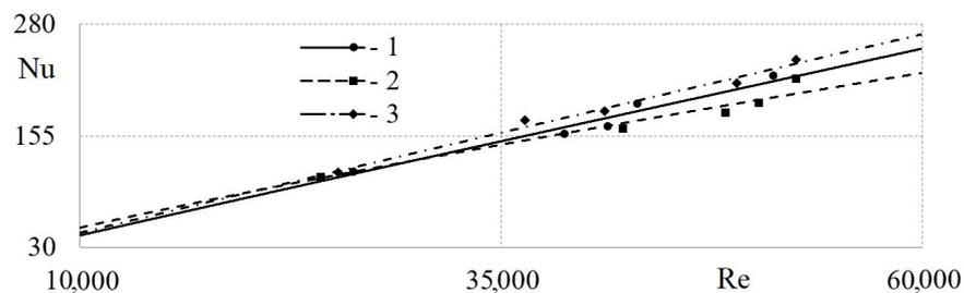
**Figure 12.** Dependences of the Nusselt number  $Nu$  on the Reynolds number  $Re$  in the intake system with channels of different diameters: 1— $d = 26$  mm; 2— $d = 32$  mm; 3— $d = 40$  mm.
