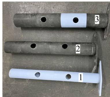
**Figure 4.** Photographs of the examined inlet pipes with different inner diameters  $d$ : 1— $d = 26$  mm; 2— $d = 32$  mm (basic configuration); 3— $d = 40$  mm.
