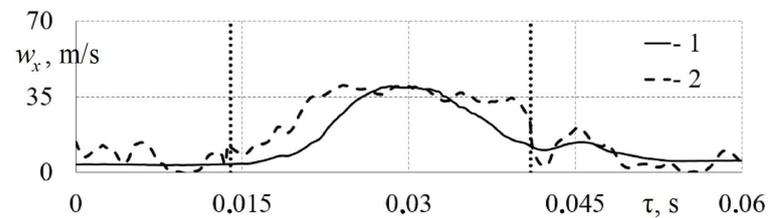
**Figure 7.** Dependences of the local ( $l_x = 100$  mm) air flow velocity  $w_x$  in the intake systems of the engine laboratory model (1) and gasoline RICE (2) on time  $\tau$  for a crankshaft speed of 1800 rpm and for  $d = 32$  mm. The vertical lines indicate the opening and closing times of the intake valve.
