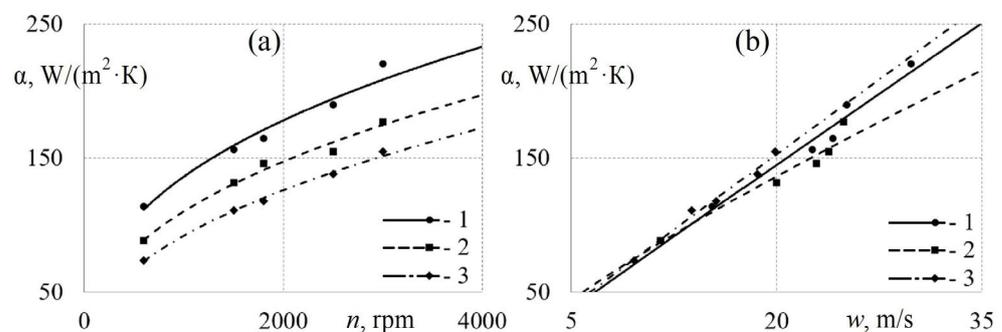
**Figure 11.** Dependences of the average heat transfer coefficient  $\alpha$  on the crankshaft speed  $n$  (a) and the average flow rate  $w$  (b) in the intake system with channels of different diameters: 1— $d = 26$  mm; 2— $d = 32$  mm; 3— $d = 40$  mm.
