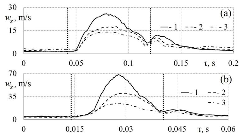
**Figure 6.** Dependences of the local ( $l_x = 100$  mm) air flow velocity  $w_x$  in the intake system of a piston engine on time  $\tau$  for crankshaft speeds of 600 rpm (a) and 1800 rpm (b) for different intake channel diameters: 1— $d = 26$  mm; 2— $d = 32$  mm; 3— $d = 40$  mm. The vertical lines indicate the opening and closing times of the intake valve.
