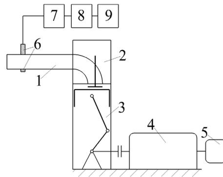
**Figure 1.** Diagram of the test bench and measuring equipment: 1—inlet channel; 2—cylinder head; 3—cylinder-piston group of the engine; 4—electric engine; 5—frequency converter; 6—hot-wire anemometer sensors (channels  $w_x$  and  $\alpha_x$ ); 7—hot-wire anemometer; 8—analogue-to-digital converter; 9—personal computer.
