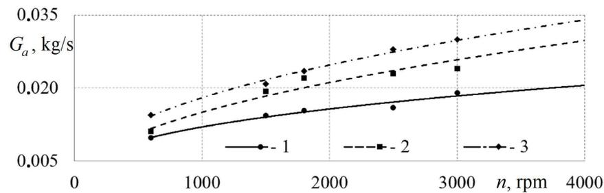
**Figure 10.** Dependences of the mass air flow  $G_a$  on the crankshaft speed  $n$  through the intake system with channels of different diameters: 1— $d = 26$  mm; 2— $d = 32$  mm; 3— $d = 40$  mm.
