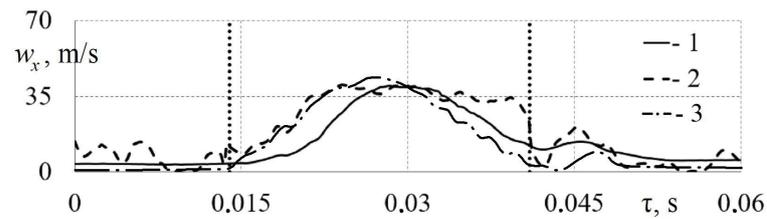
**Figure 13.** Dependences of the local air flow velocity  $w_x$  in the intake systems of the engine laboratory model (1), gasoline RICE (2), and mathematical model (3) on time  $\tau$  for a crankshaft speed of 1800 rpm and for  $d = 32$  mm. The vertical lines indicate the opening and closing times of the intake valve.
