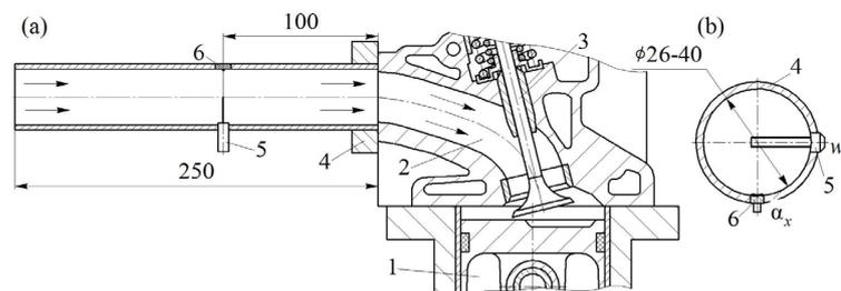
**Figure 2.** Diagram of the intake system (a) and cross section of the control section (b) (arrows indicate the air flow direction): 1—piston; 2—supply channel; 3—head of the engine pack; 4—inlet pipe; 5—speed sensor; 6—thermal sensor.
