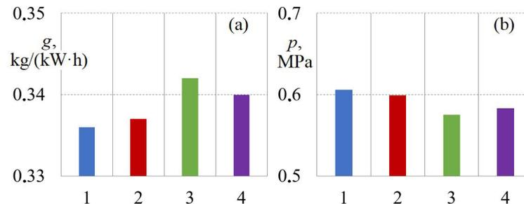
**Figure 15.** Diagrams of values of specific fuel flow  $g$  (a) and average cycle pressure  $p$  (b) of the engine in nominal mode for an intake system with channels of different diameters: 1— $d = 20$  mm; 2— $d = 32$  mm; 3— $d = 40$  mm; 4— $d = 50$  mm.
