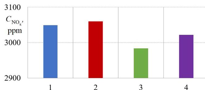
**Figure 16.** Diagrams of NO<sub>x</sub> concentration values in the exhaust gases of the engine at nominal mode for the intake system with channels of different diameters: 1— $d = 20$  mm; 2— $d = 32$  mm; 3— $d = 40$  mm; 4— $d = 50$  mm.
