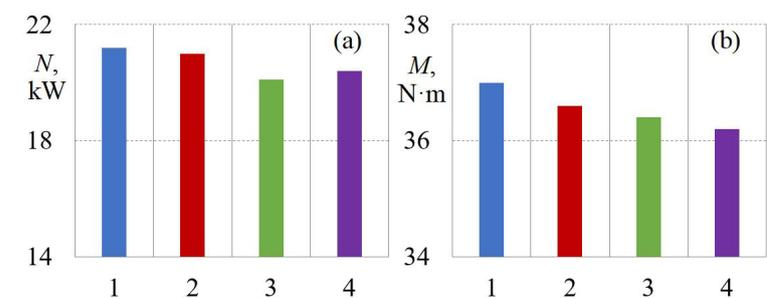
**Figure 14.** Diagrams of nominal power  $N$  (a) at  $n = 5600$  rpm and maximum torque  $M$  (b) at  $n = 4000$  rpm for an intake system with channels of different diameters: 1— $d = 20$  mm; 2— $d = 32$  mm; 3— $d = 40$  mm; 4— $d = 50$  mm.
