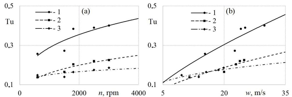
**Figure 9.** Dependences of the degree of turbulence Tu of the flows on the crankshaft speed  $n$  (a) and the average flow velocity  $w$  (b) in the intake system with channels of different diameters: 1— $d = 26$  mm; 2— $d = 32$  mm; 3— $d = 40$  mm.
