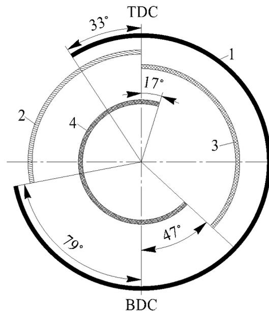
**Figure 3.** Valve timing for this study: 1—intake process; 2—compression process; 3—expansion process; 4—exhaust process; TDC—top dead centre; BDC—bottom dead centre.
