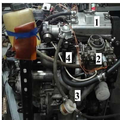
**Figure 5.** Gasoline engine for verification of laboratory research data and modelling results: 1—engine block head; 2—inlet pipeline; 3—exhaust manifold; 4—cylinder block.
