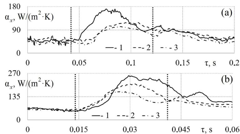
**Figure 8.** Dependences of the local ( $l_x = 100$  mm) heat transfer coefficient  $\alpha_x$  in the intake system of a piston engine on time  $\tau$  for crankshaft speeds of 600 rpm (a) and 1800 rpm (b) for different diameters of the intake channel: 1— $d = 26$  mm; 2— $d = 32$  mm; 3— $d = 40$  mm. The vertical lines indicate the opening and closing times of the intake valve.
