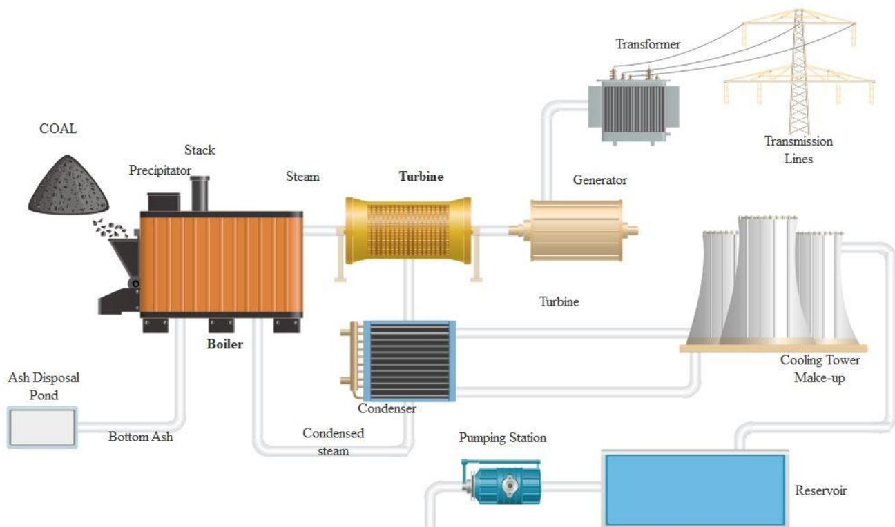
**Figure 2.** Schematic of the coal-fired TPP representing major equipment [22].
