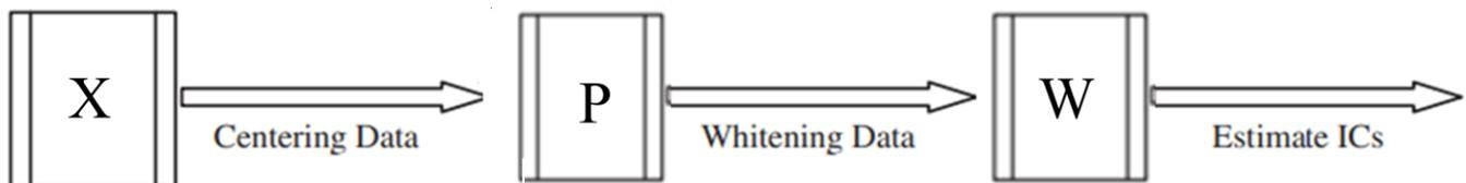
**Figure 8.** Illustration of the Mixing and Separation Process using ICA Algorithm [96].
