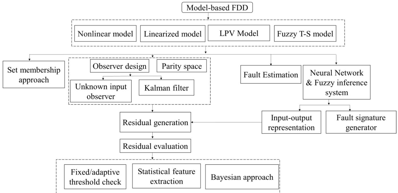
Figure 5. Illustration of Model-Based Fault Detection TPP Systems.
