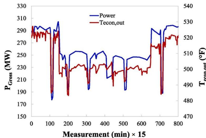
**Figure 9.** Consequence of a Leak: A Graph Showing the Decrease in Economizer Outlet Temperature [101].
