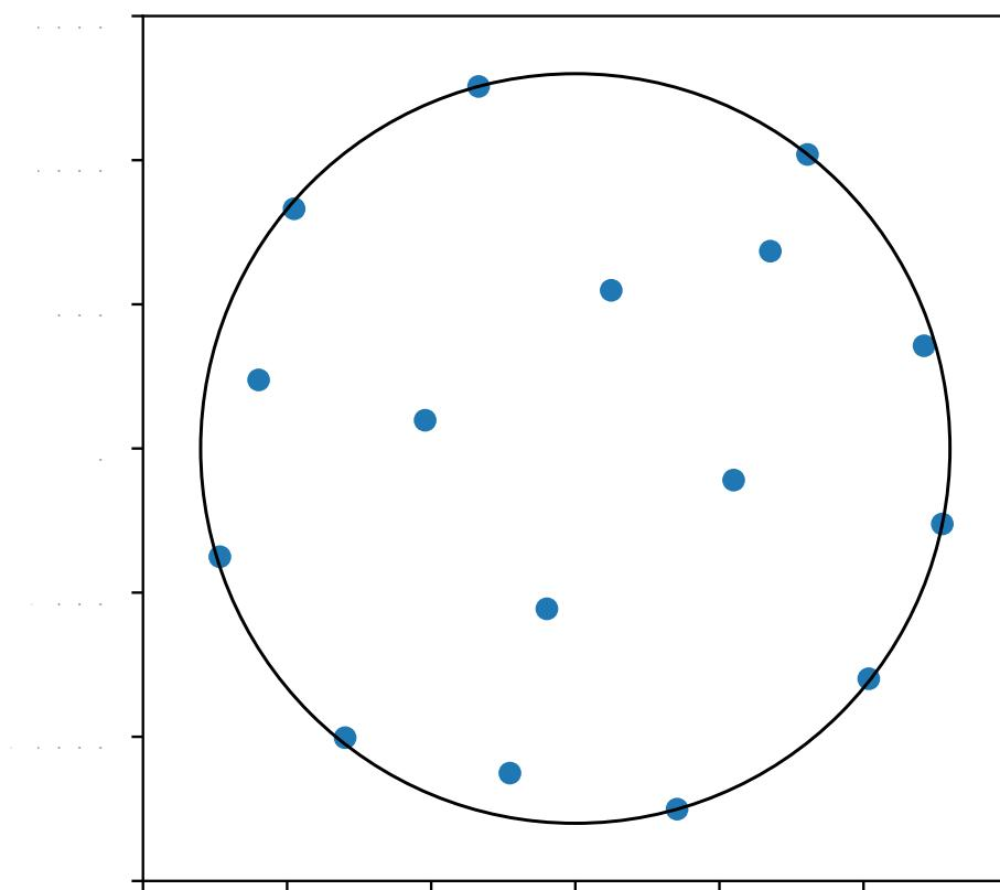
**Figure 6.** Turbine layout by means of DPCRO-SL (16 turbines, 1300m radius).
