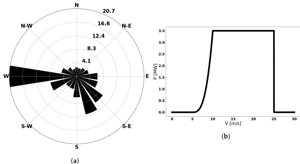
**Figure 5.** (a) Wind rose of the challenge [55]. (b) Power curve of the NREL's 3.35-MW onshore reference turbine [55].
