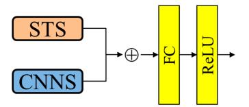
Figure 3. The fusion structure of the output features of Swin Transformer stem and CNN stem.
