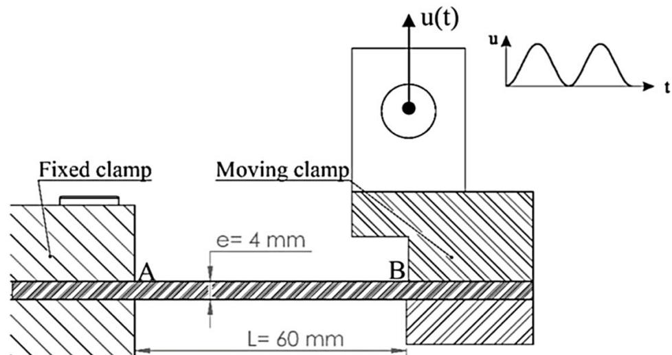
Figure 1. Specimen clamping.
