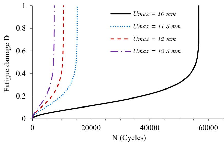
Figure 15. Simulated damage evolution at the extreme fixed outer layer of PA66GF20 specimens.
