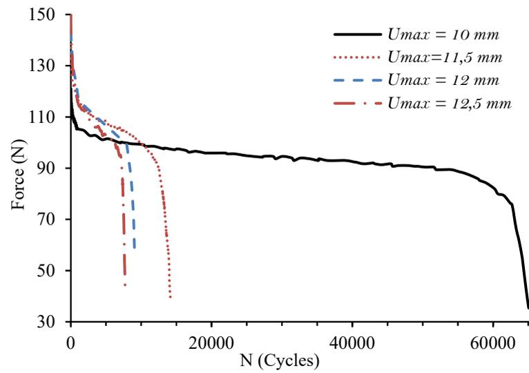
Figure 11. Experimentally measured force-cycle history for PA66GF20 specimens.
