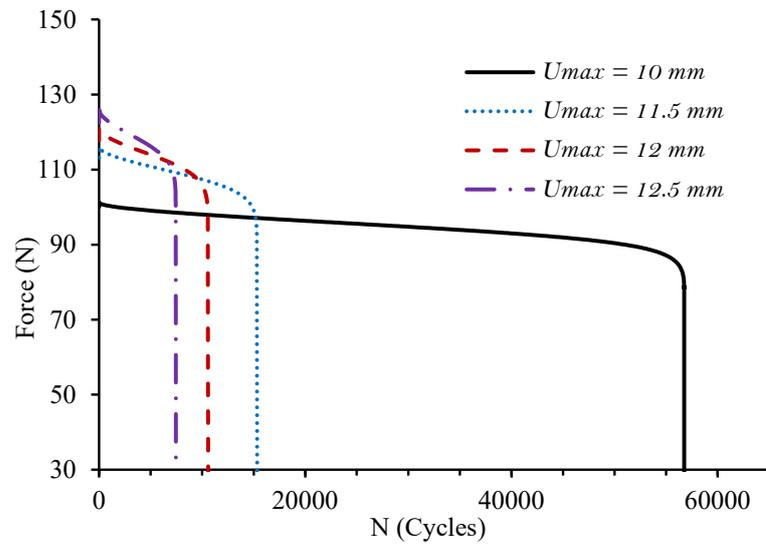
Figure 13. Simulated force-cycle history for PA66GF20 specimens.
