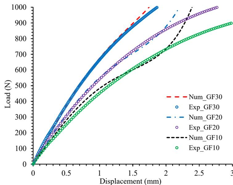
Figure 3. Load-displacement curves of tensile tests on PA66GFs: transverse direction.
