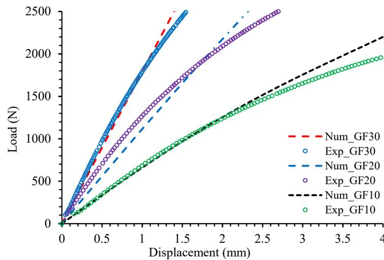
Figure 2. Load-displacement curves of tensile tests on PA66GFs: longitudinal direction.
