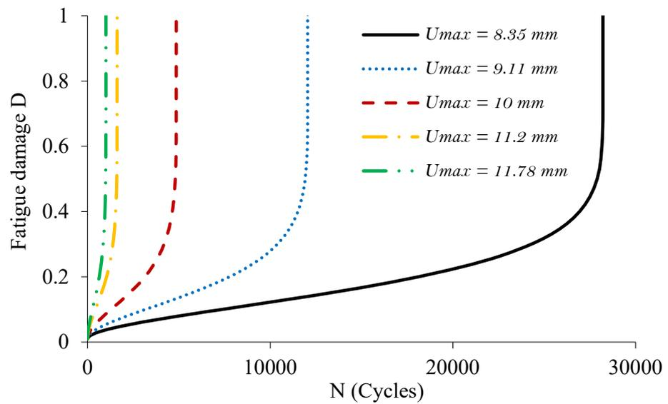
Figure 16. Simulated damage evolution at the extreme fixed outer layer of PA66GF30 specimens.
