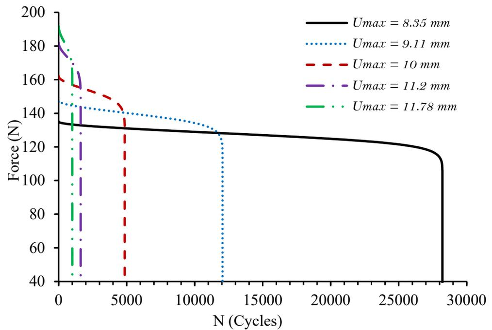
Figure 14. Simulated force-cycle history for PA66GF30 specimens.
