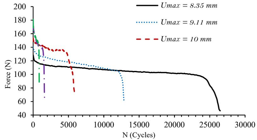
Figure 12. Experimentally measured force-cycle history for PA66GF30 specimens.
