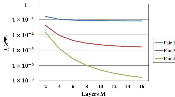
**Figure 4.** Three graphs of the dependence of the minimum value  $J_i^{opt} = J_i(\mathbf{e}^{opt})$  of the cost functional  $J_i$  corresponding to the shielding problem on the number of isotropic layers  $M$  for three different pairs  $(\varepsilon_{\min}, \varepsilon_{\max})$  given in (31).
