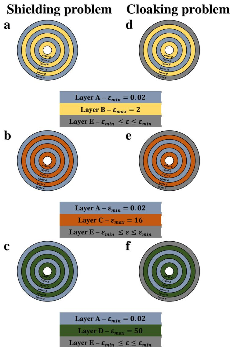
**Figure 5.** Schematic of optimal six-layered isotropic shells obtained when solving shielding (a–c) or cloaking (d–f) problems for three different pairs  $(\epsilon_{min}, \epsilon_{max})$  given in (31) [the first pair—(a,d); the second pair—(b,e); the third pair—(c,f)].
