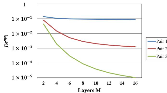
**Figure 6.** Three graphs of the dependence of the minimum value  $J^{opt} \equiv J(\mathbf{e}^{opt})$  of the cost functional  $J$  corresponding to the cloaking problem on the number of isotropic layers  $M$  for three different pairs  $(\epsilon_{\min}, \epsilon_{\max})$  given in (31).
