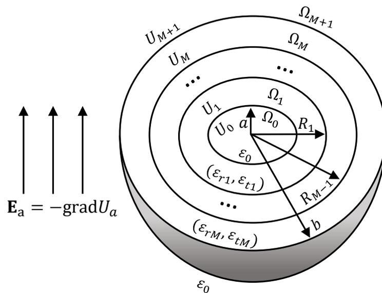
**Figure 1.** Schematic representation of an externally applied electric field  $\mathbf{E}_a$  and the multilayer spherical shell  $(\Omega, \epsilon)$ , immersed in free space.
