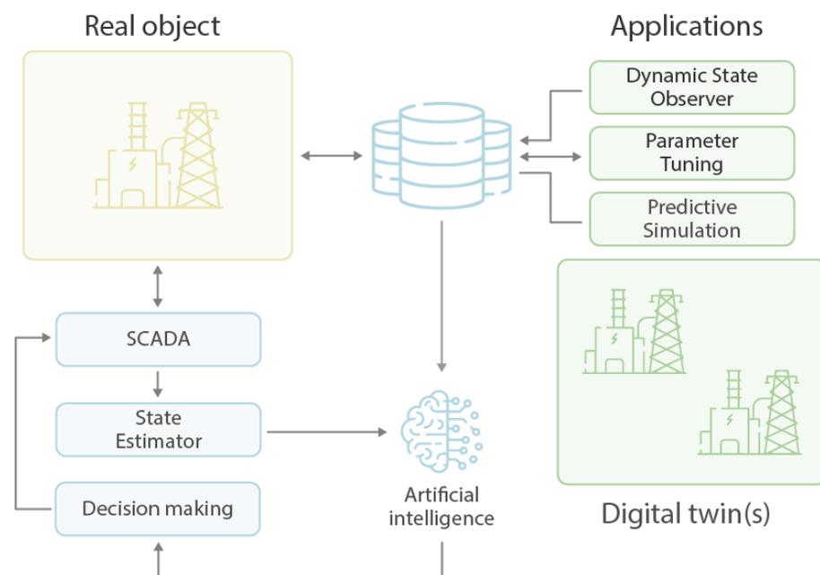
**Figure 5.** Digital twin architecture for the real object control system.
