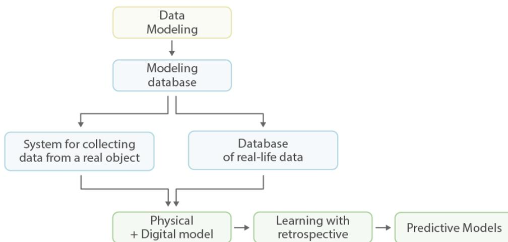
**Figure 4.** The main elements of the digital twin model for power equipment life cycle management.
