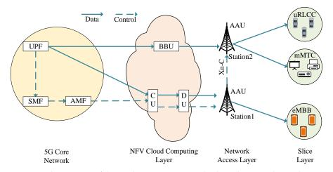
Figure 1. The structure of the two base stations serve the three slices together under CU-DU separation.
