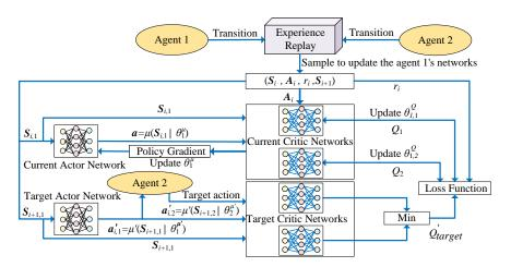
Figure 3. The training process of MATD3 in optimizing the upper level resource allocation problem.
