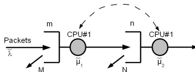
Figure 2. Queuing system representation for the case of one single processor.
