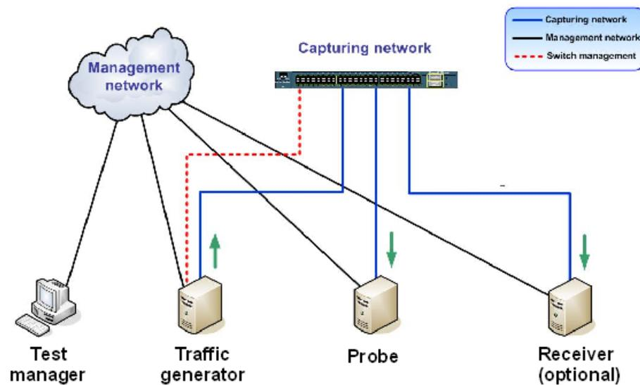
Figure 3. Testbed platform for experimental measurements.
