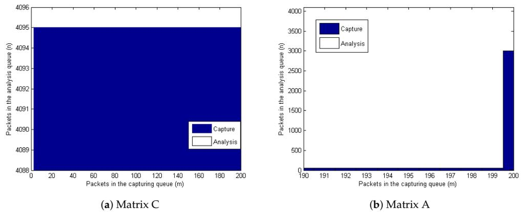
Figure 5. Optimal policy with network traffic rate of 620,000 pps and null analysis load.
