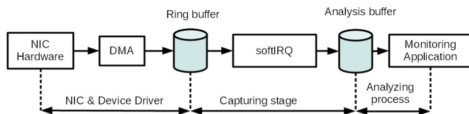
**Figure 1.** Packet receiving process with Linux networking subsystem.
