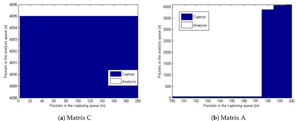
Figure 4. Optimal policy with network traffic rate of 100,000 pps and null analysis load.
