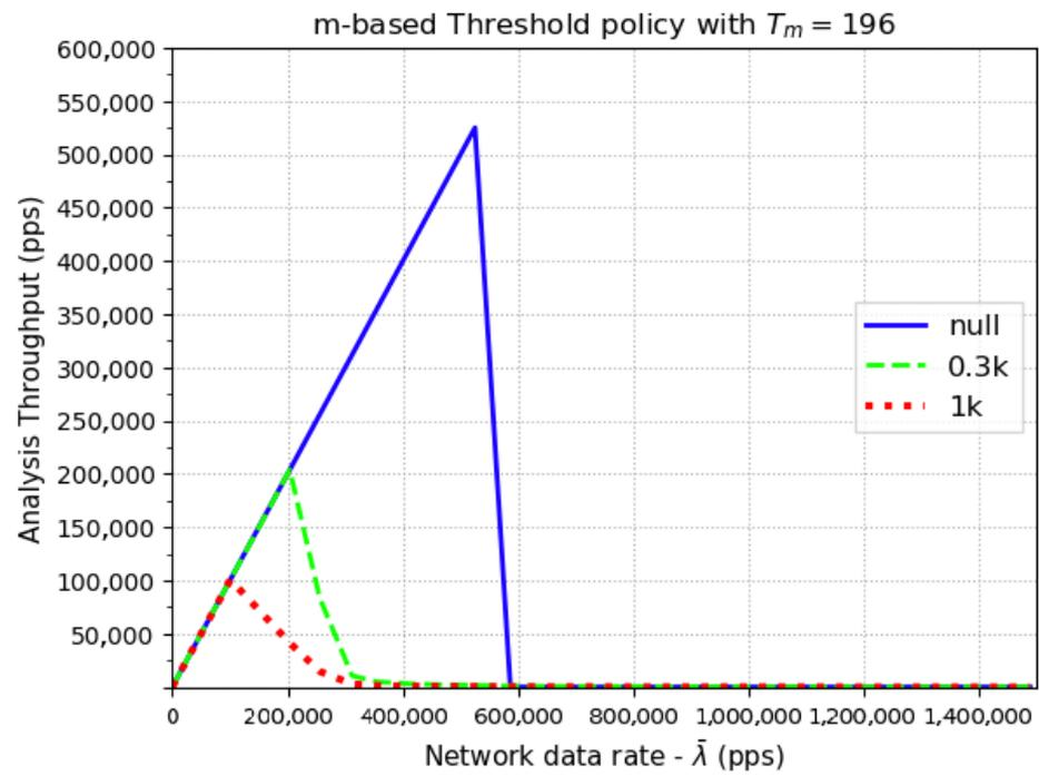
Figure 9. Performance simulation for m-based threshold policy.
