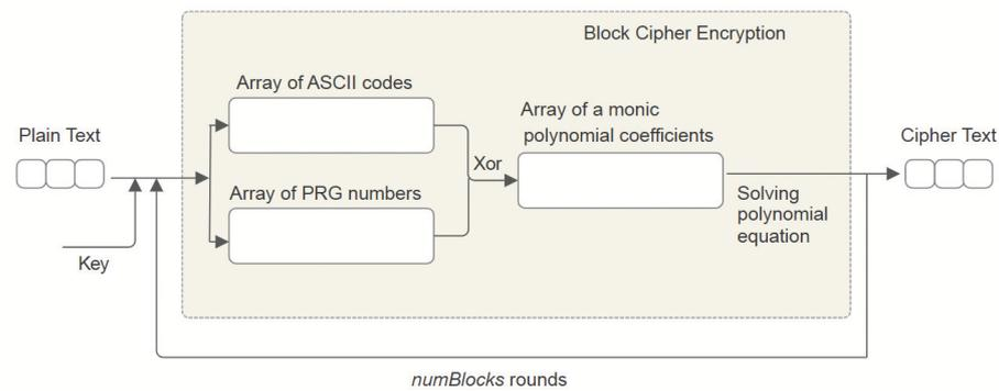
Figure 2. Encryption scheme.
