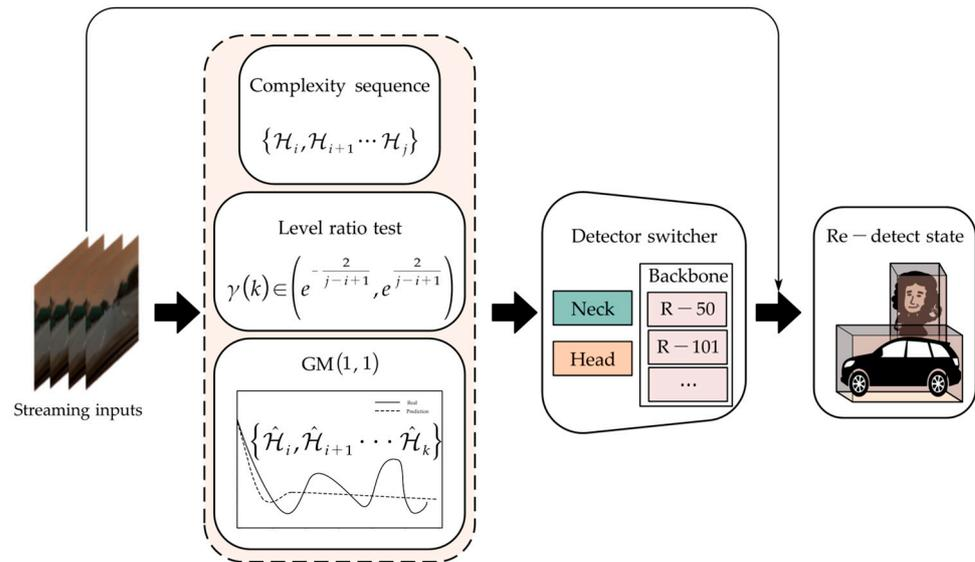
**Figure 6.** The streaming input updating switcher, where the GM (1, 1) is utilized to predict the future complexity of streaming inputs and is used as a basis for switching the backbone structure in the detector switcher and updating the re-detect state.
