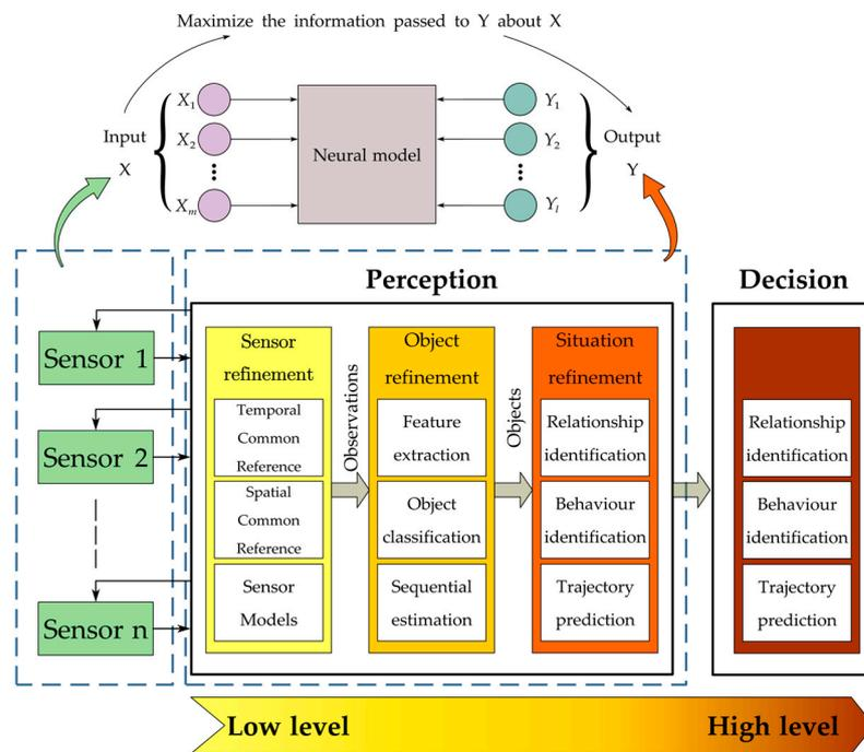
**Figure 2.** The perception system process encompasses various levels of data, information processing, and modeling in an overall scheme. We view the sensor’s inputs and perceived performance in the model as the I/O of the streaming.
