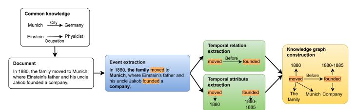
Figure 1. General pipeline for event-centric temporal knowledge graph construction.
