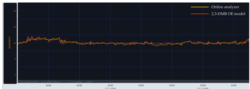
Figure 14. The 2,3-DMB content OE model implementation results in the real plant [51].
