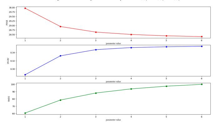
**Figure 12.** The trend of PSNR, DV–BV, and SMD2 for fusion images with the increase in fusion parameters. The red line represents the variation of PSNR, the blue line represents the variation of DV-BV, and the green line represents the variation of SMD2.
