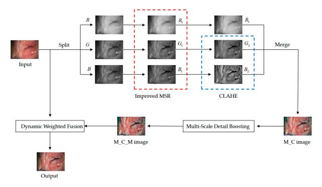
Figure 2. Overall flowchart of the proposed algorithm.
