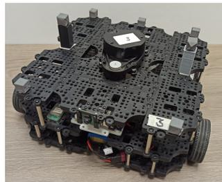
**Figure 3.** Turtlebot3<sup>®</sup> Waffle Pi. Onboard cubes of silver reflective fabric are used for tracking purposes.
