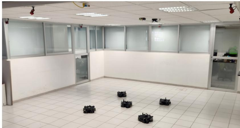
**Figure 4.** OptiTrack<sup>®</sup> setup for real-world implementations. The six cameras Flex3<sup>®</sup> are installed on the ceiling.
