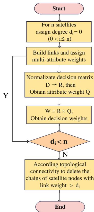
Figure 3. The flowchart of MCOTG algorithm.
