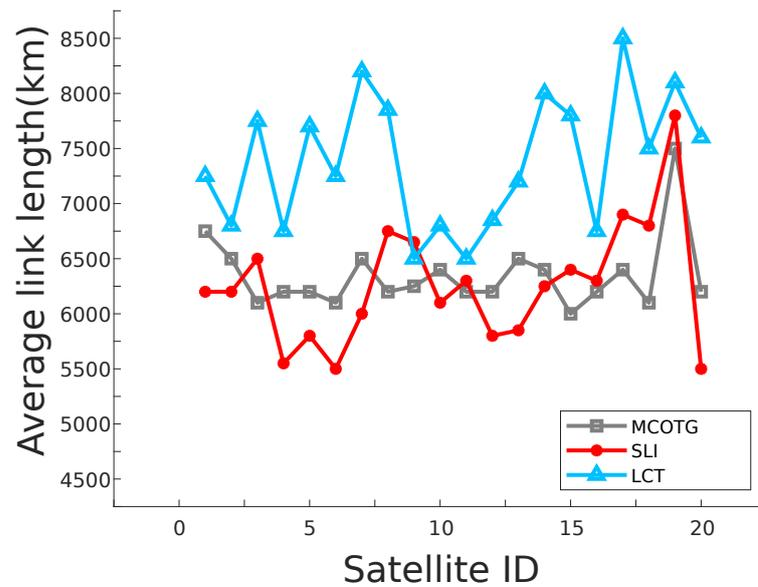
**Figure 6.** Comparison of average link length in network topology.
