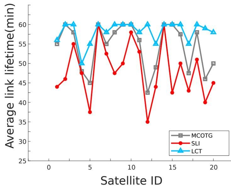
Figure 8. Comparison of average link lifetime in network topology.
