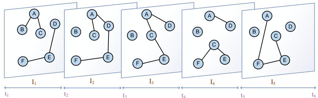
Figure 1. The topology time-varying diagram of constellation satellite network.
