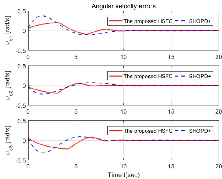
Figure 12. Comparison of angular velocity tracking errors.
