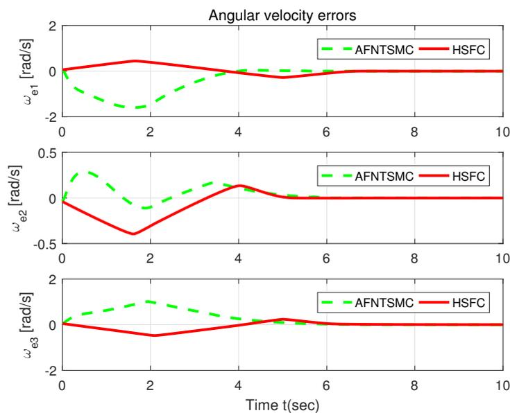
Figure 8. Comparison of angular velocity tracking errors.
