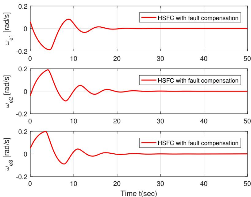
Figure 5. Angular velocity tracking errors.
