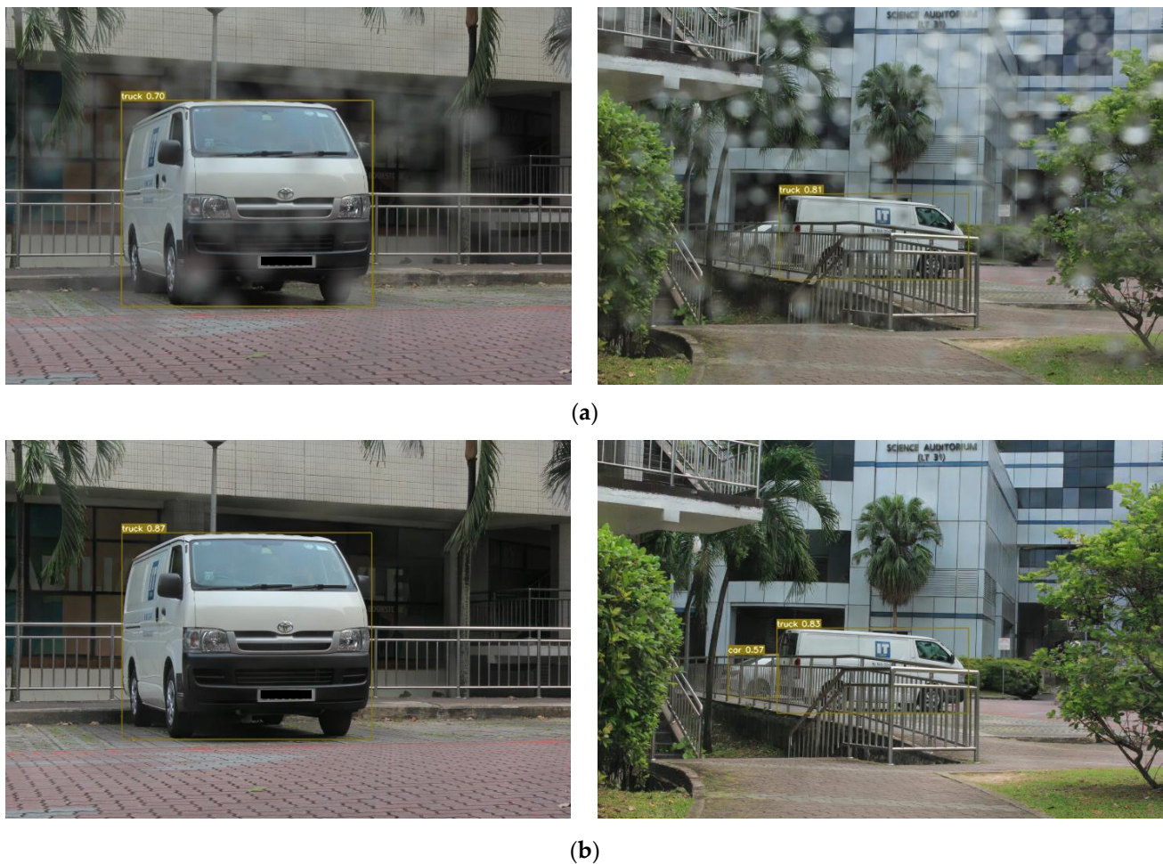
Figure 15. The results of the object detection (YOLOv7) for the raindrop and raindrop-removal images. (a) raindrop images; (b) proposed raindrop-removal images.
