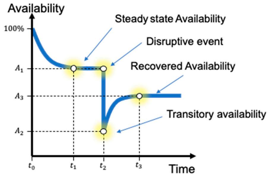
Figure 2. System availability subject to degradation and shock (adapted from [12]).
