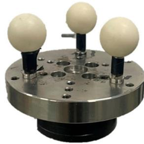
Figure 4. Calibration plate. (Physical image).
