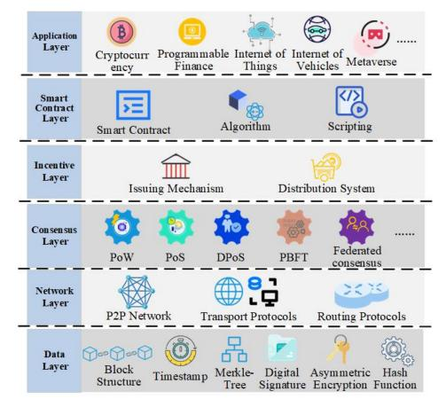
Figure 2. The basic architecture of blockchain.
