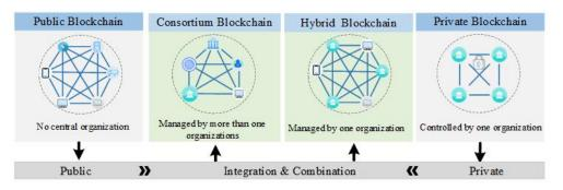
Figure 3. The four types of blockchain.
