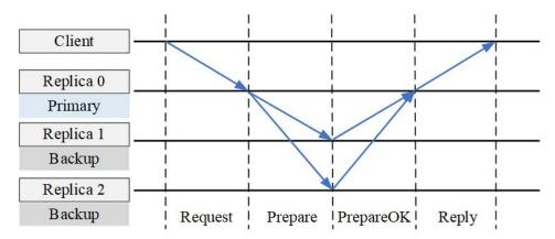
Figure 6. The consistency process of the VR mechanism in a normal case.
