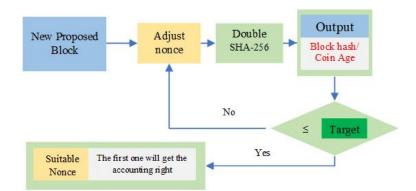
Figure 13. The process of random number search in PPcoin PoS consensus mechanism.
