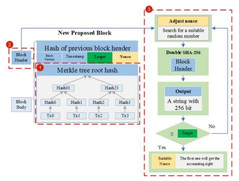
determines the required calculation amount for this puzzle. The process of random number search in the Bitcoin PoW consensus mechanism is shown in Figure 12.
