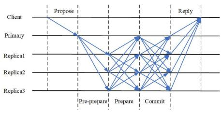
Figure 11. The phases of the PBFT.
