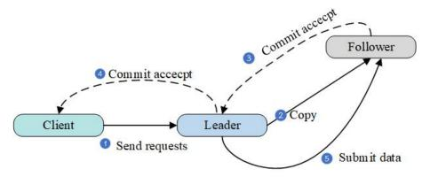
Figure 10. The process of Raft log replication.
