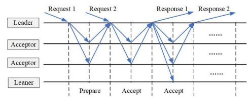
Figure 8. The flow of the Multi Paxos mechanism.
