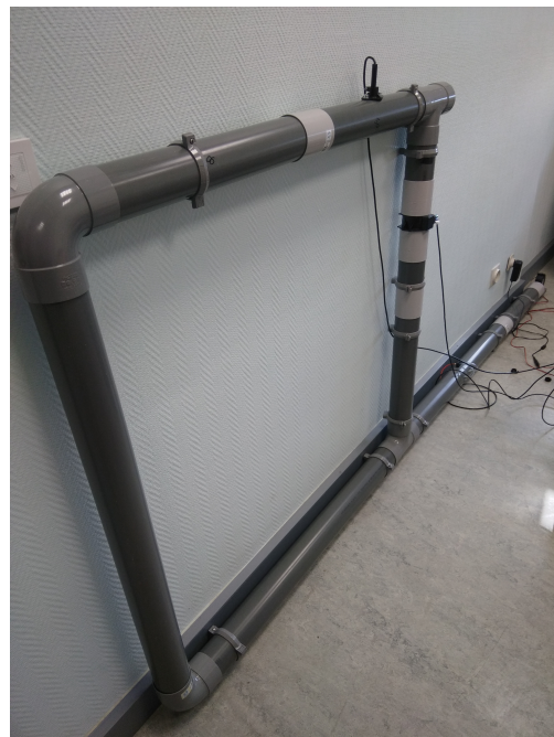
Figure 6. Experimental set-up of a ventilation network: The benchmark is built to emulate conditions in a typical small mine, a scale 1:500 has been used in order to configure the crosssection of the tunnels.
