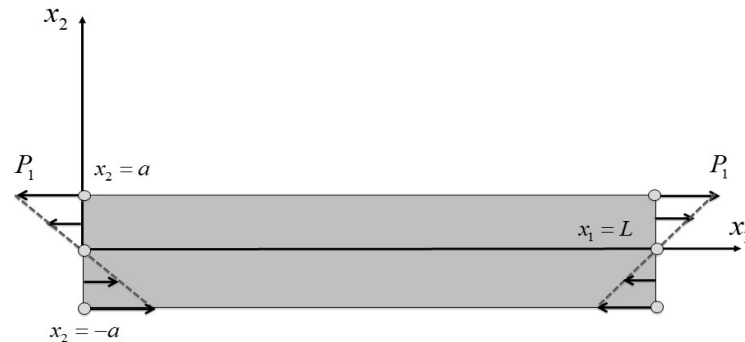
Figure 1. Pure bending of an elastic beam.
