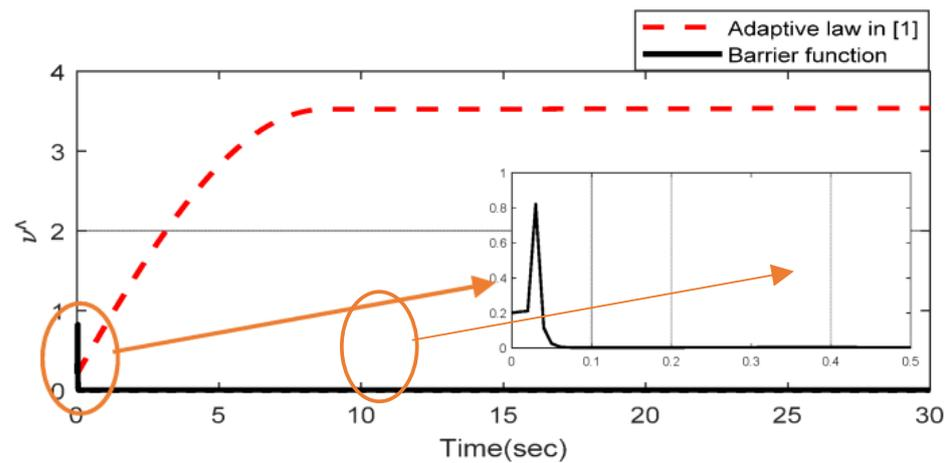
Figure 5. Time responses of the barrier function and adaptive law.
