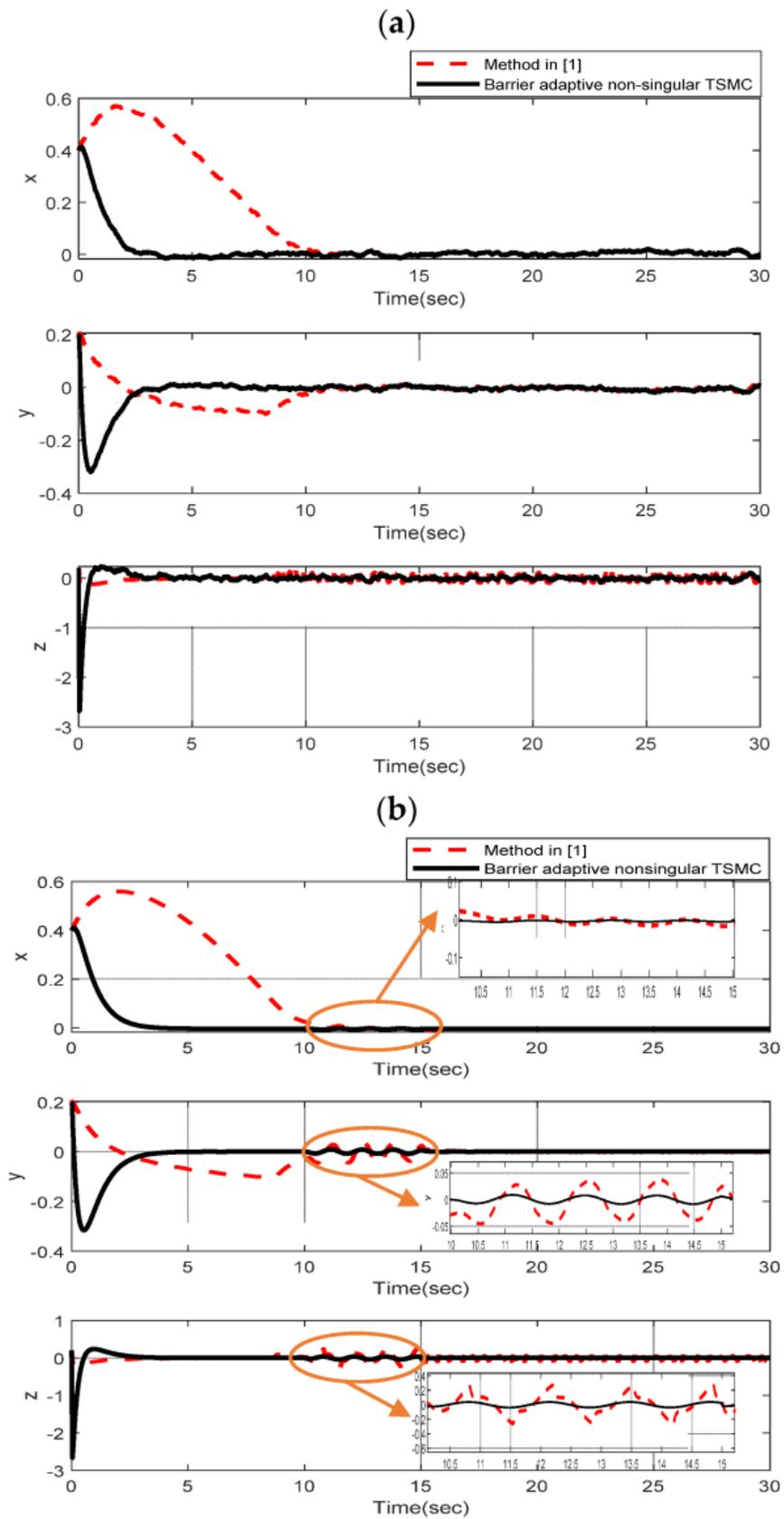
**Figure 7.** State trajectories of a system (a) with noise (b) in the presence of an abrupt change in disturbance.
