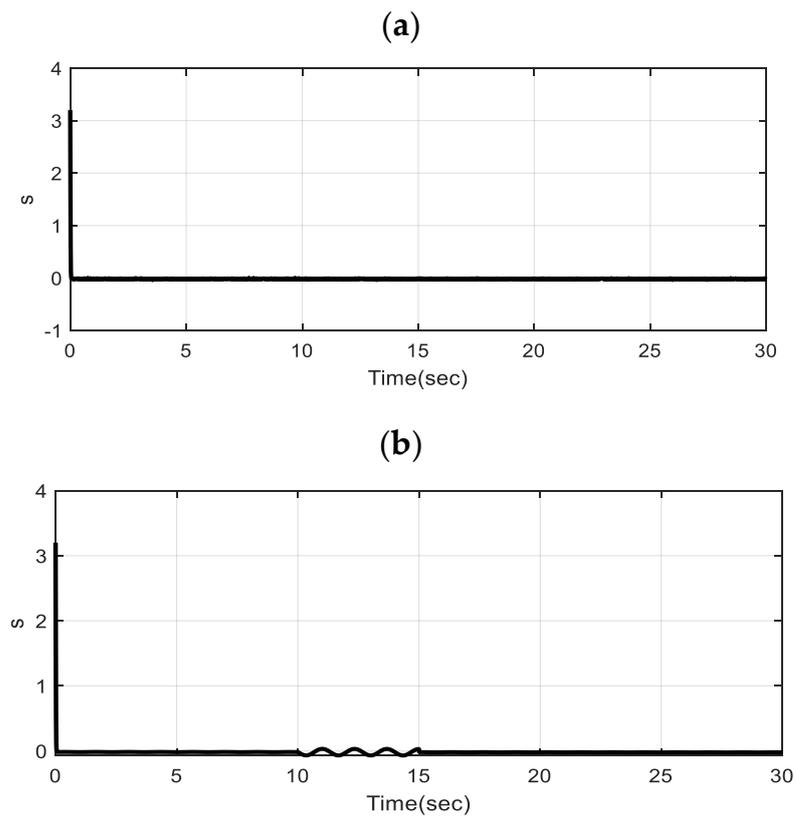
Figure 8. Time histories of a nonlinear sliding surface (a) with noise (b) in the presence of an abrupt change in disturbance.
