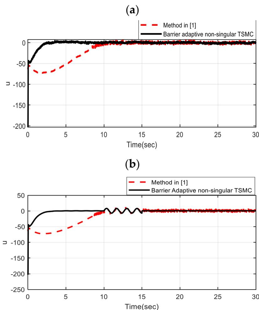
**Figure 10.** Trajectory of control inputs (a) with noise (b) in the presence of an abrupt change in disturbance.
