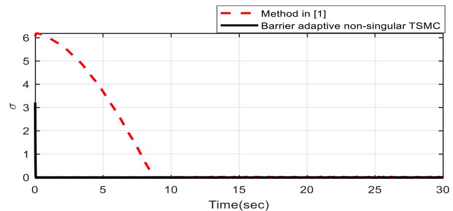
Figure 4. Time responses of the non-singular terminal sliding surface.
