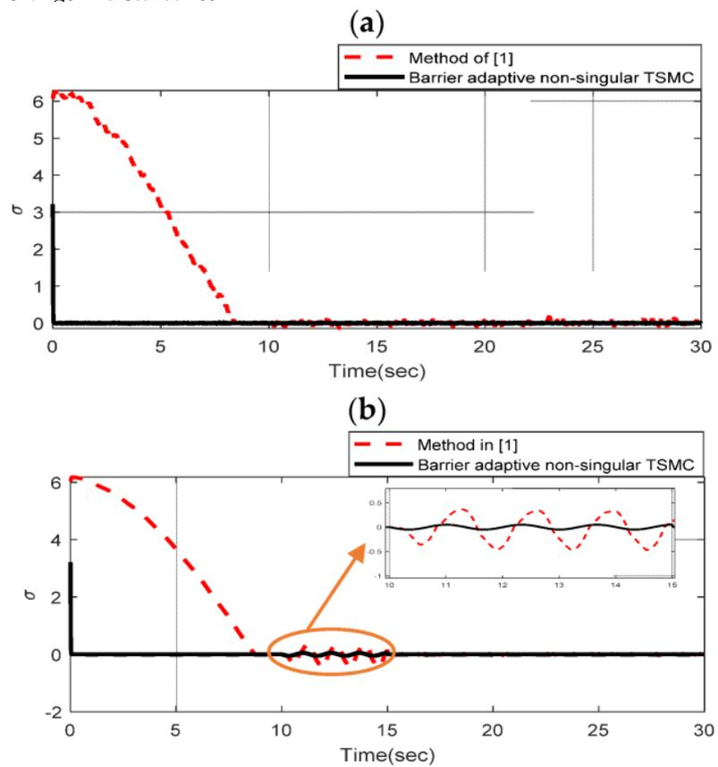
Figure 9. Time responses of a non-singular terminal sliding surface (a) with noise (b) in the presence of abrupt change in disturbance.
