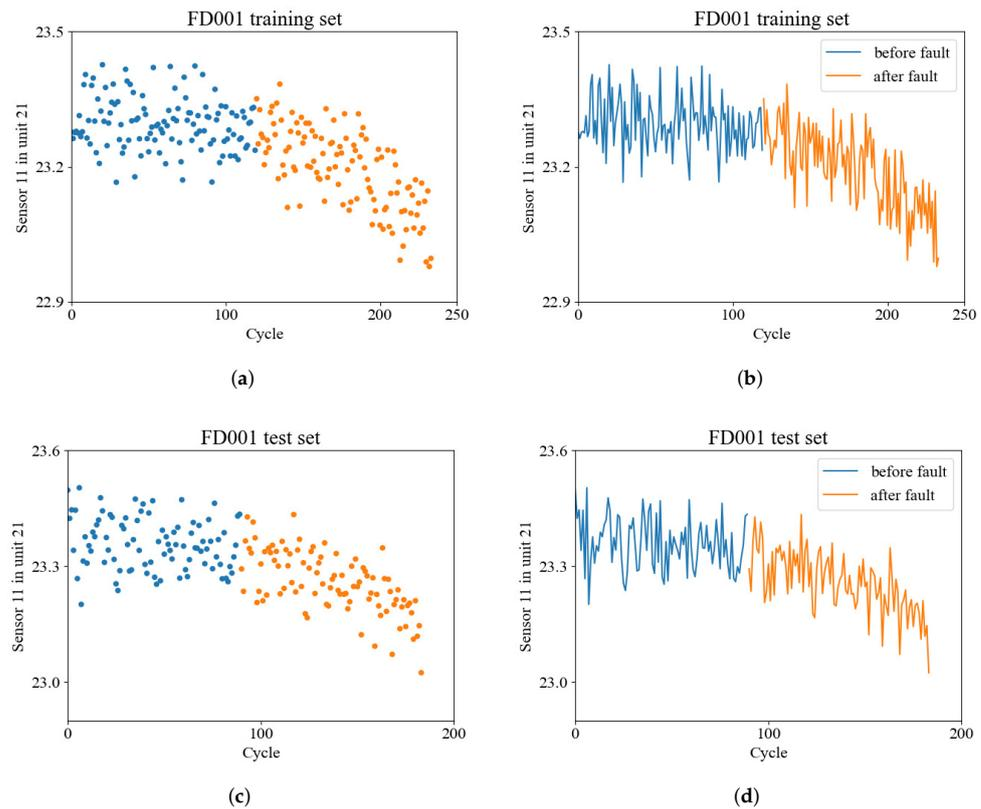
**Figure 4.** Fault detection using k-means. (a) K-means scatter plot; (b) Fault detection in training set; (c) K-means scatter plot; (d) Fault detection in test set.
