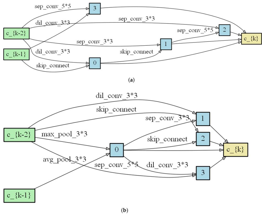
**Figure 5.** Architectures learned on C-MAPSS. (a) normal cell; (b) reduction cell.
