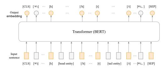
**Figure 3.** The feature encoder of our proposal. Orange items represent special mark tokens, e.g., [CLS] and [SEP] are the start and end of the input sentence with  $L_x$  words, and [h] ([t]) and [/h] ([/t]) are the start and end of the head entity span and tail entity span, respectively.
