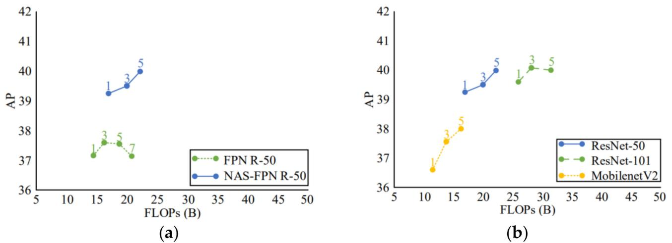
**Figure 14.** Impact of NAS-FPN on text detection. Impact of (a) search algorithm and (b) backbone network on model performance.
