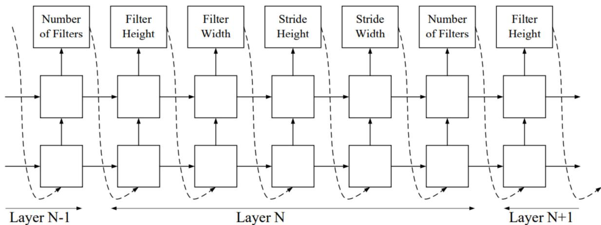
Figure 8. Predictive structure flowchart for RNN controller.
