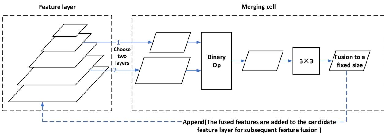
Figure 5. Structure of fusion unit.
