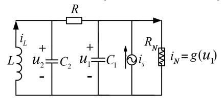
Figure 1. 3D Filippov-type slow-fast Chua's circuit diagram.
