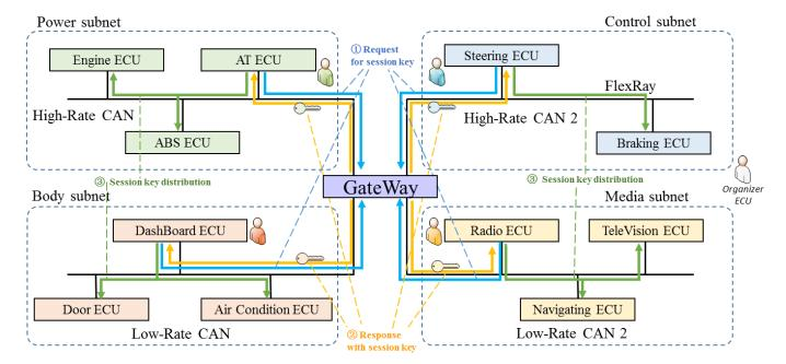
Figure 1. The structure of the in-vehicle network.
