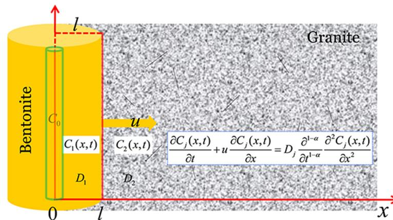
Figure 1. Deep geological disposal concept of the HLW repository.
