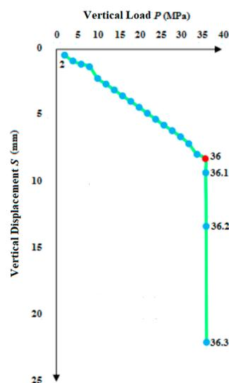
Figure 10. P-S curve is the fitting result of the numerical result in Table 2, and the red point is a sudden shift of vertical subsidence.
