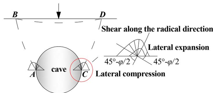
**Figure 4.** Vertical cross-section of limestone strata containing the spherical Karst cave, which was affected by the vertical load.
