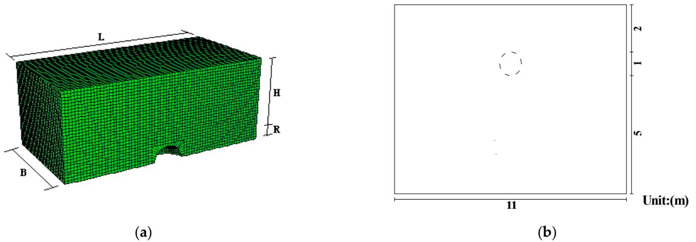
Figure 8. Sketch of numerical simulation model. (a) 1/4 geometry model, and mesh; (b) The dimensions of numerical simulation model.
