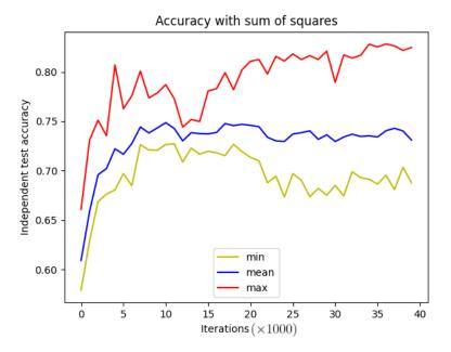
**Figure 5.** Five training results of Fashion-MNIST classification in frequency domain with the proposed nonlinear activation function, with square sum. The red color means the maximum accuracy, the yellow color is the minimum accuracy and the blue line shows the mean accuracy.
