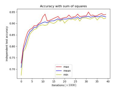
**Figure 4.** Five training results of MNIST classification in frequency domain with the proposed nonlinear activation function, with square sum instead of inverse FFT. The red color means the maximum accuracy, the blue line shows the mean accuracy and the yellow color is the minimum accuracy.
