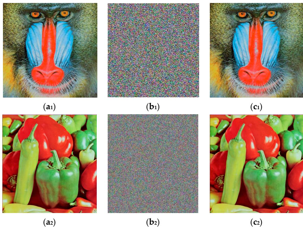
**Figure 3.** Some more standard RGB plain images along with their encrypted and decrypted versions; (a) Peppers ( $256 \times 256 \times 3$ ); (b) encrypted peppers; (c) decrypted peppers; (a<sub>1</sub>) baboon ( $256 \times 256 \times 3$ ); (b<sub>1</sub>) encrypted baboon; (c<sub>1</sub>) decrypted baboon; (a<sub>2</sub>) peppers ( $512 \times 512 \times 3$ ); (b<sub>2</sub>) encrypted peppers; (c<sub>2</sub>) decrypted peppers.
