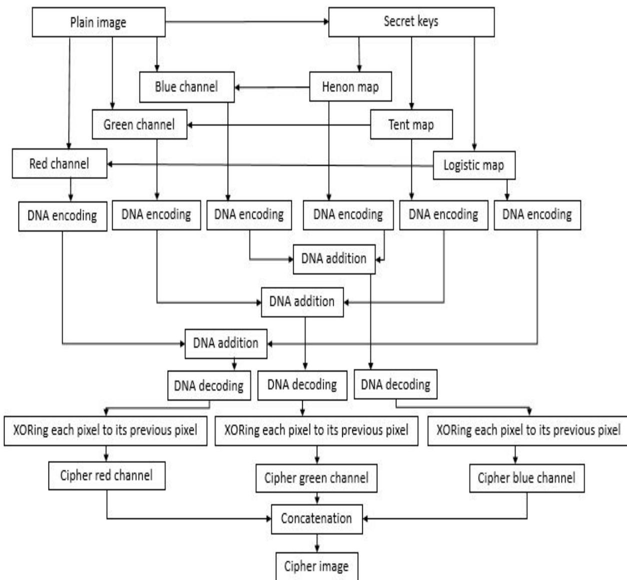
**Figure 1.** Block diagram of the proposed encryption scheme.
