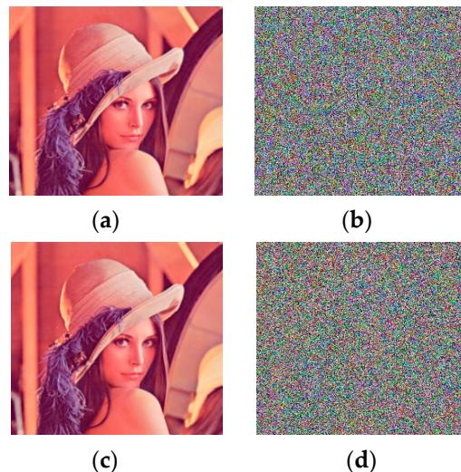
**Figure 4.** Key sensitivity analysis of Lena ( $256 \times 256 \times 3$ ). (a) Plain RGB Lena; (b) encrypted Lena using a set of keys; (c) decrypted Lena using a correct set of keys; (d) decrypted Lena by bringing a minor change in one of the keys.
