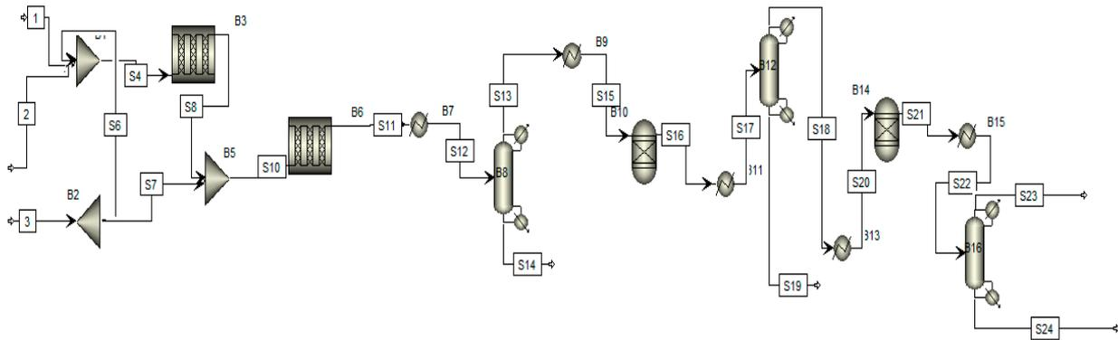
**Figure 2.** Process flow diagram of the Claus process.
