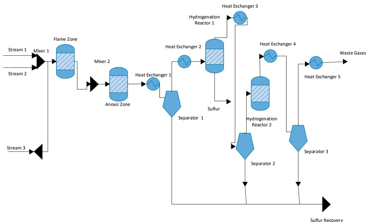
**Figure 1.** Block Flow diagram of the Claus process.
