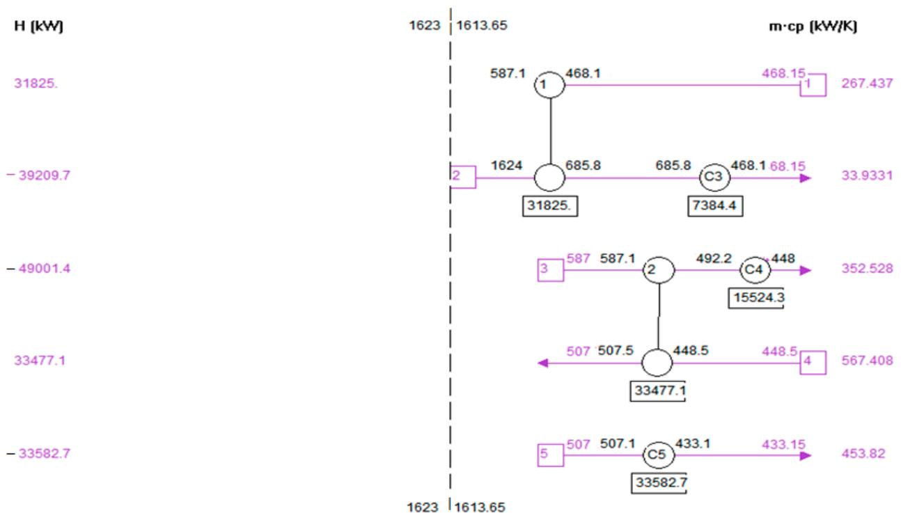
Figure 8. Heat exchanger network (HEN) design of heat exchanger.
