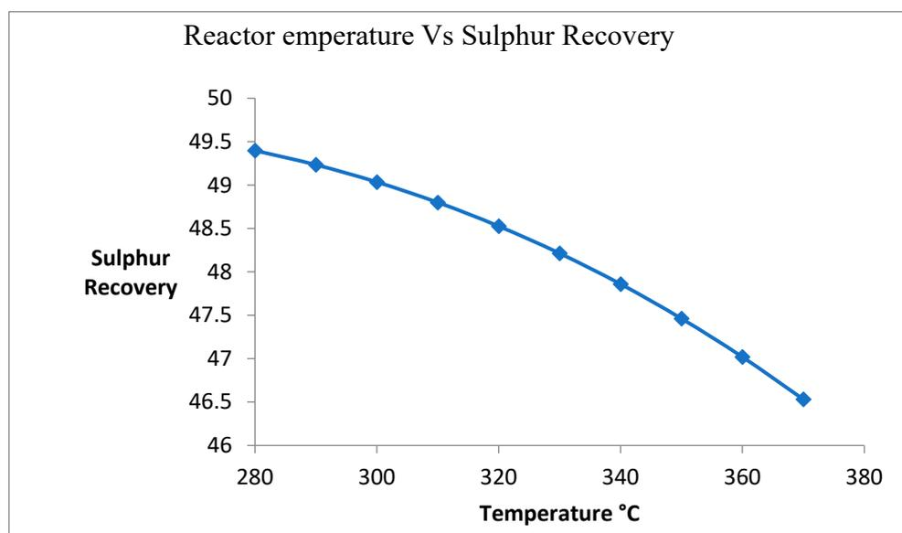
Figure 5. Effect of change in temperature on sulfur recovery.
