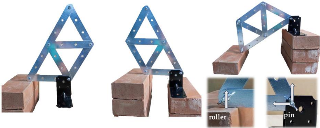
Figure 8. Warren-type truss supported in various ways, using a roller and a pin.
