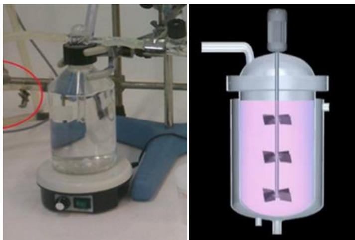
**Figure 3.** Real continuous stirred tank reactor (left), and raw digital flow model resource (right).
