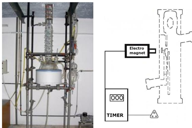
**Figure 4.** Capture of the downside of the pilot plant batch distiller (left), and AR marker for the reflux splitter device.
