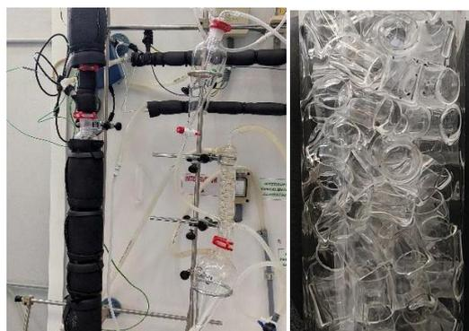
**Figure 5.** Bottom of the distillation column body (**left**), and still image of the distillation column inside (**right**).
