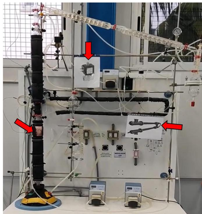
**Figure 7.** Continuous Distillation experimental equipment with the three markers created.
