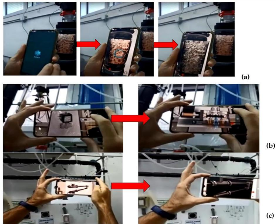
**Figure 6.** Different moments during the implementation and launch of the AR-based teaching tool. (a) Inner flow into the column; (b) Operation of the reflux valve; (c) Flow into the heat exchanger.
