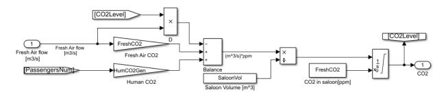
**Figure 6.** Model of the CO<sub>2</sub> signal.
