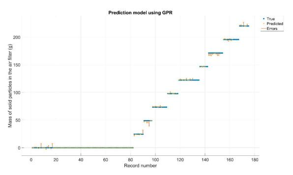
Figure 9. Response of the Gaussian process regression model after validation process.
