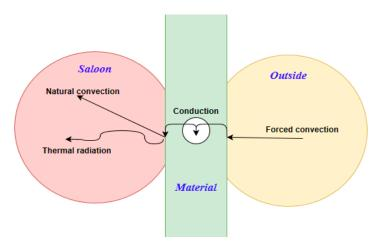
Figure 7. Types of heat transfer through materials.
