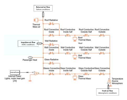
Figure 5. Model of the cabin thermal networking.
