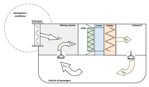
Figure 8. Ventilation system, circulation of air flow.
