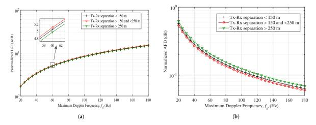
**Figure 4.** Level-crossing-rate (LCR) and average fade duration (AFD) plotted against different values of maximum Doppler shift in (**a**,**b**), respectively; for different scenarios of outdoor mmWave (case 1; 38 GHz) radio propagation environments. (m = 1,  $\rho = 2$ ).
