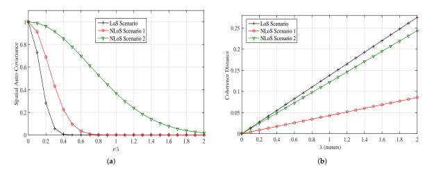
**Figure 11.** Spatial auto-covariance and CD for different scenarios of indoor mmWave (Case 3; 28 GHz) radio propagation environments in (**a**,**b**), respectively. (m = 4 for LoS Scenario and m = 1 for NLoS Scenarios,  $f_d = 10$  Hz).
