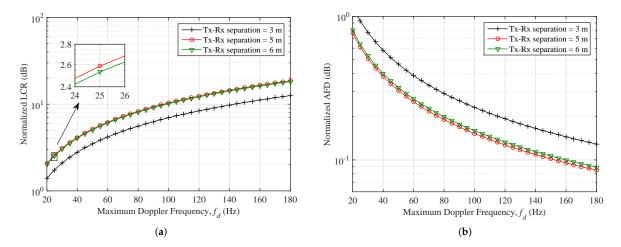
**Figure 6.** LCR and AFD plotted against different values of maximum Doppler shift in (a,b), respectively; for different scenarios of indoor mmWave (Case 2 (a); 28 GHz) radio propagation environments.  $(m = 1, \rho = 2)$ .
