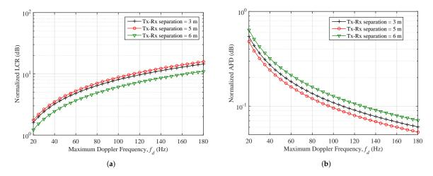
**Figure 8.** LCR and AFD plotted against different values of maximum Doppler shift in ( $\mathbf{a}$ , $\mathbf{b}$ ), respectively; for different scenarios of indoor mmWave (Case 2 (b); 38 GHz) radio propagation environments. ( $m = 1, \rho = 2$ ).
