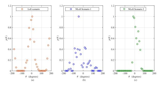
**Figure 3.** Angular distribution of multipath power with respect to azimuth AoA for different indoor mmWave (28 GHz) radio propagation environments; obtained after performing numerical integration along delay domain, data calibrations, and normalization operations on the measurement results provided in [6]. (a) LoS Scenario, Figure 8b of [6]; (b) NLoS Scenario 1, Figure 8e of [6]; (c) NLoS Scenario 2, Figure 8h of [6].
