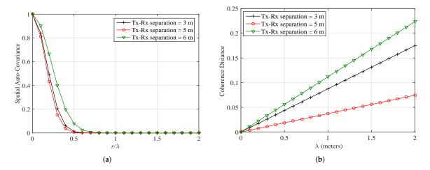
**Figure 9.** Spatial auto-covariance and CD for different scenarios of indoor mmWave (Case 2 (b); 38 GHz) radio propagation environments in (**a**,**b**), respectively. (m = 1,  $f_d = 10$  Hz).
