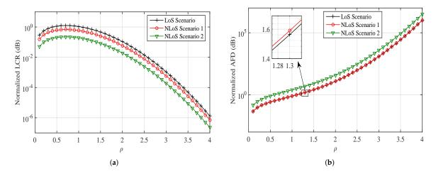
**Figure 10.** LCR and AFD plotted against different values of threshold levels in ( $\mathbf{a}$ , $\mathbf{b}$ ), respectively; for different scenarios of indoor mmWave (Case 3; 28 GHz) radio propagation environments. (m = 4 for LoS Scenario and m = 1 for NLoS Scenarios,  $f_d = 1$  Hz).
