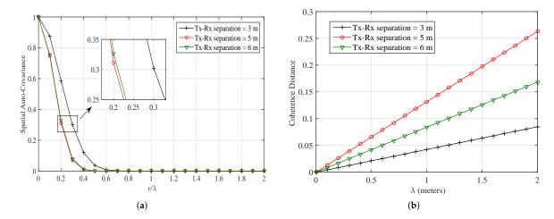
**Figure 7.** Spatial auto-covariance and CD for different scenarios of indoor mmWave (Case 2 (a); 28 GHz) radio propagation environments in ( $\mathbf{a}$ , $\mathbf{b}$ ), respectively. (m = 1,  $f_d = 10$  Hz).
