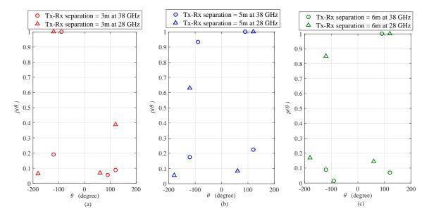
**Figure 2.** Angular distribution of multipath power with respect to azimuth AoA for different mmWave (38 GHz and 28 GHz) indoor corridor environments; obtained after data calibrations, and normalization operations performed on the measurement results provided in [7]. (a) Tx-Rx separation = 3 m; (b) Tx-Rx separation = 5 m; (c) Tx-Rx separation = 6 m Figure 13 of [7].
