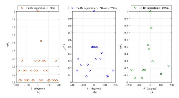
**Figure 1.** Angular distribution of multipath power with respect to azimuth angle of arrival (AoA) for different outdoor mmWave (38 GHz) radio propagation environments; obtained after data calibrations, and normalization operations performed on the measurement results provided in [4]. (a) Tx-Rx separation < 150 m; (b) Tx-Rx separation > 150 and < 250 m; (c) Tx-Rx separation > 250 m Figure 7 of [4].
