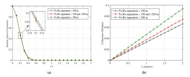
**Figure 5.** Spatial auto-covariance and coherence distance (CD) for different scenarios of outdoor mmWave (case 1; 38 GHz) radio propagation environments in ( $\mathbf{a}$ , $\mathbf{b}$ ), respectively. (m = 1,  $f_d = 1$  Hz).
