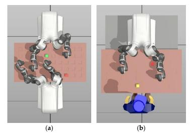
**Figure 2.** Pick-and-place scenario with: (**a**) two collaborative ABB YuMi robots (IRB 14,000); (**b**) one collaborative robot and a human operator sharing the workspace.
