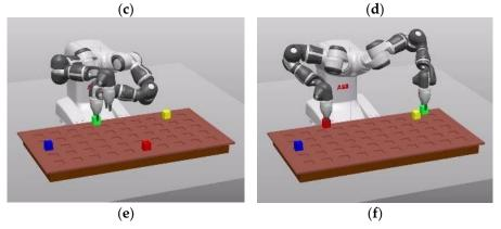
**Figure 11.** Simulation of a pick-and-place operation with Navigation Mode 4 movements (movements in 3 different heights). (a) t = 3 s; (b) t = 6 s; (c) t = 8 s; (d) t = 14 s; (e) t = 16 s; (f) t = 20 s.
