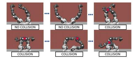
Figure 6. Visual representation of situations of collision detection.
