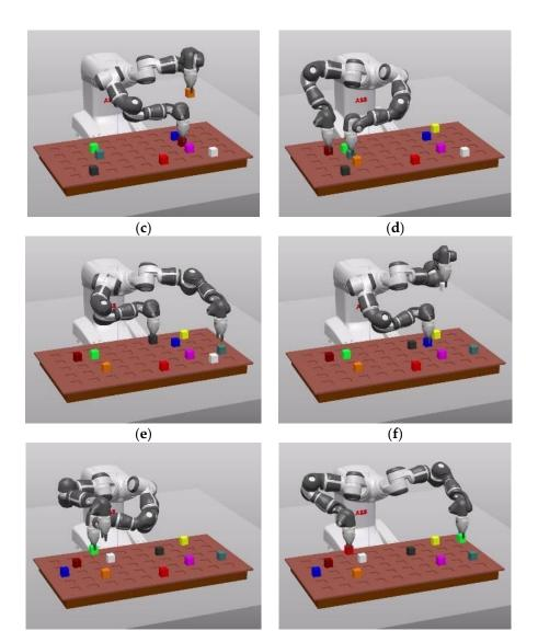
**Figure 12.** Simulation of a pick-and-place operation solved with the PDDL algorithm for 10 pieces. (a) t = 3 s; (b) t = 8 s; (c) t = 12 s; (d) t = 18 s; (e) t = 24 s; (f) t = 28 s; (g) t = 35 s; (h) t = 40 s.
