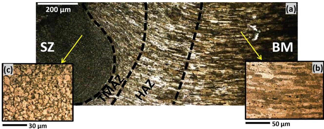
**Figure 8.** Microstructure of the grain distribution in the cross section of the AA1100 FSW weld (processed at 1120 rpm and 250 mm/min); (a) general view of the cross section, (b) the base metal, and (c) the stirring zone (SZ), at higher magnification.
