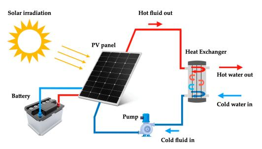
Figure 10. Schematic representation of a typical photovoltaic/thermal system.
