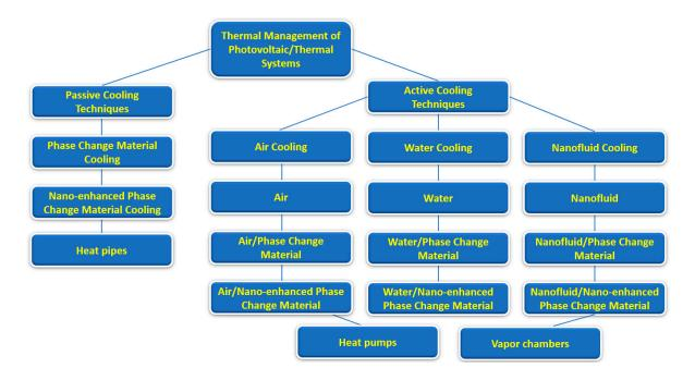
Figure 2. Main passive and active cooling techniques for photovoltaic/thermal systems.
