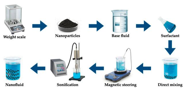
Figure 3. Typical two-step preparation method for nanofluids.
