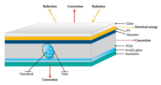
**Figure 14.** Typical configuration of a photovoltaic thermal system operating simultaneously with nanofluids and PCMs.
