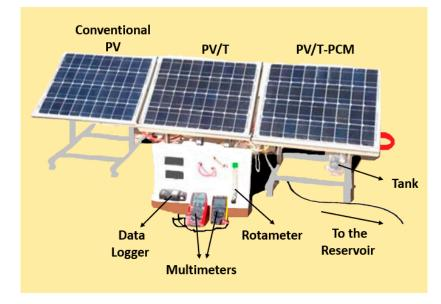
**Figure 15.** General view of the experimental setup developed by the authors Sardarabadi et al. Adapted from [135].
