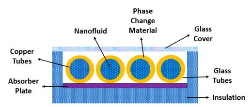
Figure 9. Configuration of the photovoltaic/thermal system. Adapted from [126].
