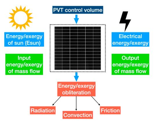
Figure 11. Energy and exergy of the control volume of a photovoltaic/thermal system.
