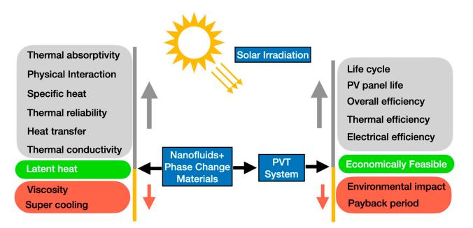
**Figure 13.** Main design parameters for a photovoltaic/thermal system operating with nanofluids and PCMs.
