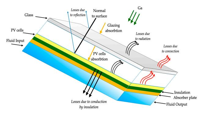
Figure 12. Main heat transfer mechanisms associated with a photovoltaic/thermal system.
