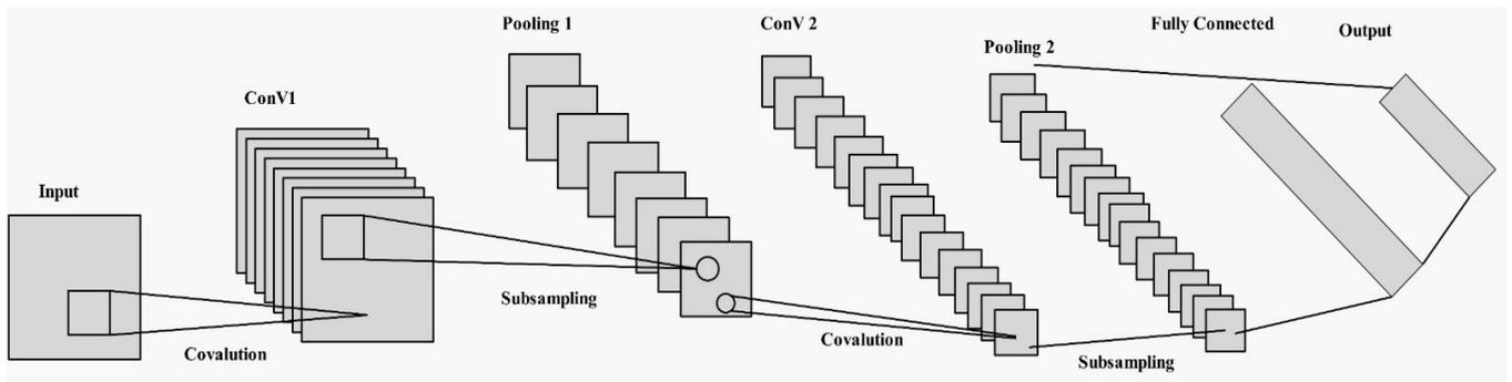
Figure 4. Architecture of the CNN model [42].
