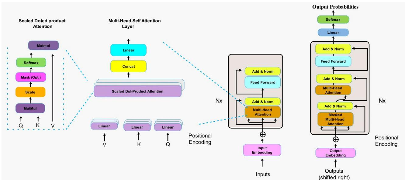
**Figure 6.** Architecture of the transformer model [45].
